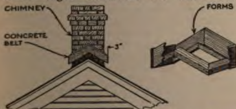
A Concrete Belt Placed around the Chimney will, Except in Very Stormy Weather, Keep Water from Leaking through the Roof along the Chimney
